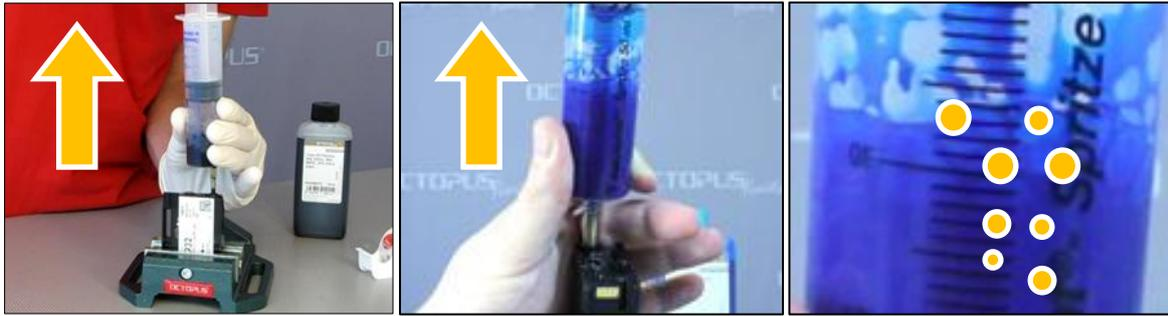
Pull up the plunger of the syringe and keep it in this upper position for one to two seconds. This creates negative pressure inside the cartridge. You can see that air bubbles arise through the refill ink inside the syringe.
